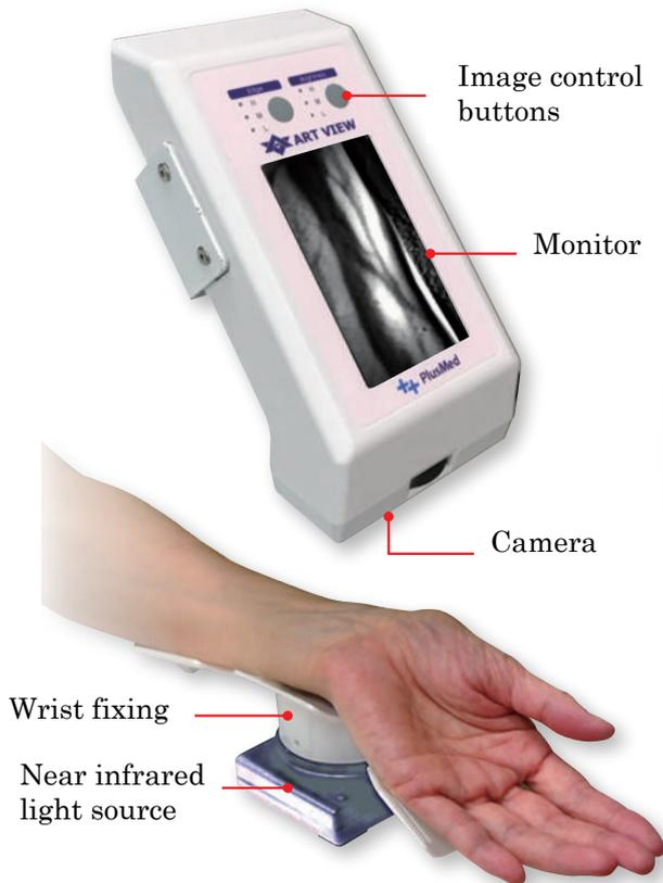
Near-infrared light projected under a wrist penetrates a hand. The information is captured by a camera above, processed and projected in real time on a monitor. Absorbed the light by hemoglobin in blood creates blood patterns in black.
